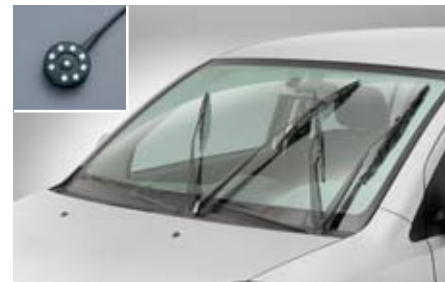
22 Rain sensor SEWAYA1000 E Activates wiper blades automatically.
